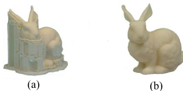
Figure 3: Support material before (a) and after removal (b). Reproduced from [2].
