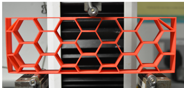
Figure 16: Photograph showing a 5% beam mounted on the Instron machine.
